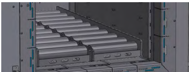
Roller conveyor in furnace chamber for heavy charges (similar to picture)
