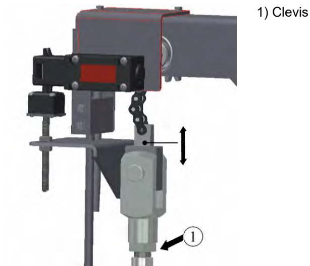
Fig. 27: Readjusting (tension) the chain (similar to picture)
